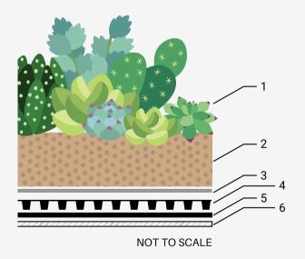
\*OVERALL DEPTH WILL INCLUDE AN ADDITIONAL 1/4 INCH FOR THE DRAINAGE SYSTEM AND A 1/2 INCH OR MORE FOR SEDUM MATS OR INTENSIVE PLANTINGS.
